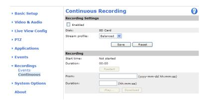
If using an SD card, the Axis product can be configured to continuously save video to the card. To prevent the disk from becoming full, it is recommended to enable automatic disk cleanup under System Options > Storage.
